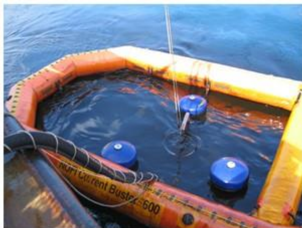
Mechanical skimmers working inside boom. Source: U.S. Coast Guard, Credit: Patrick Kelley
