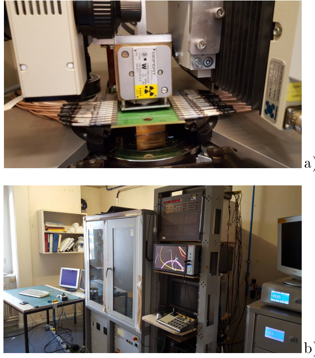
Figure 5.2: (a) 10keV X-ray source and 32-channel probe card mounted on a temperature- controlled prober at CERN. (b) Complete setup with the cabinet for irradiation experiments in the center, Keithley SCS 4200 semiconductor characterization system and switching matrix with temperate controller to right
