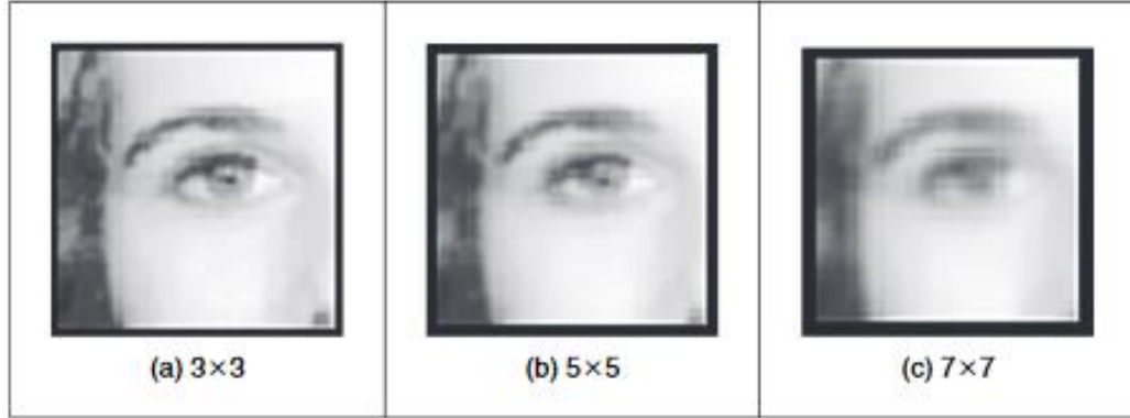
Figure 4.28: Application of Gaussian blurring by applying a (a) 3x3 kernel, (b) 5x5 kernel and (c) 7x7 kernel [92].
