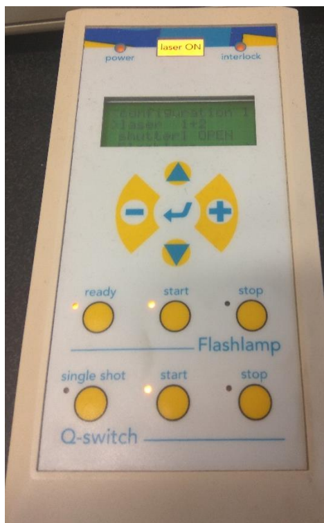
Figure B.5: Photograph of the Remote Controller, when the Flashlamp and the Q-switch are both turned on.
