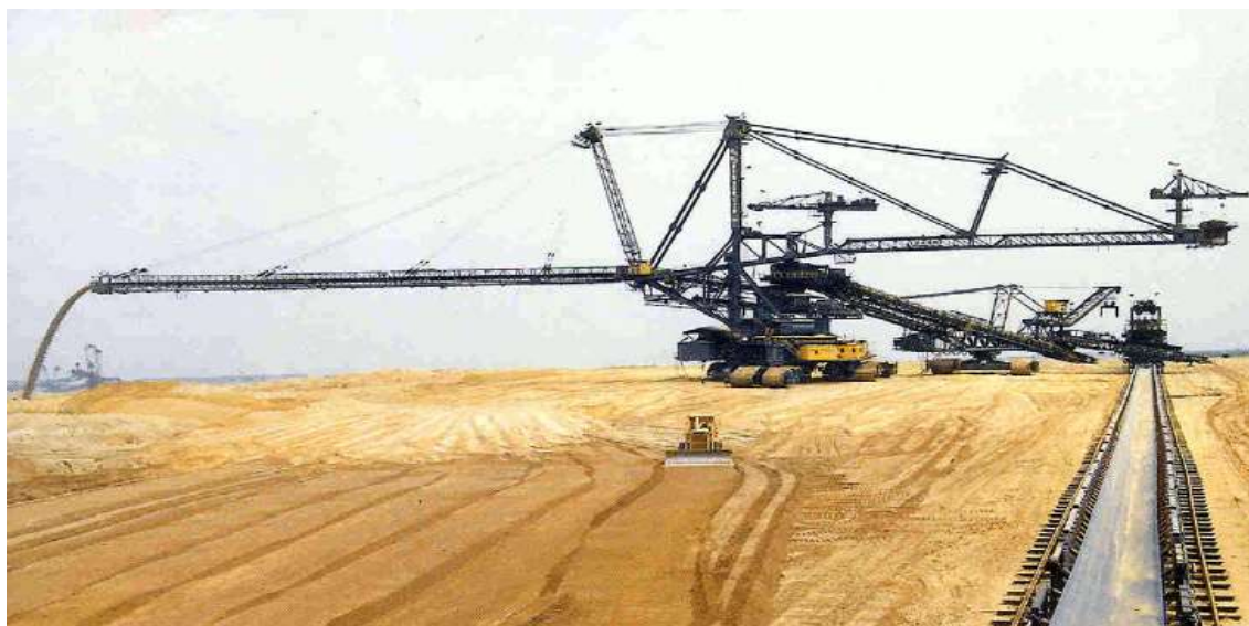
Figure 2.2: Stacking method - Stacker in operation [Steiakakis et al., 2009].
