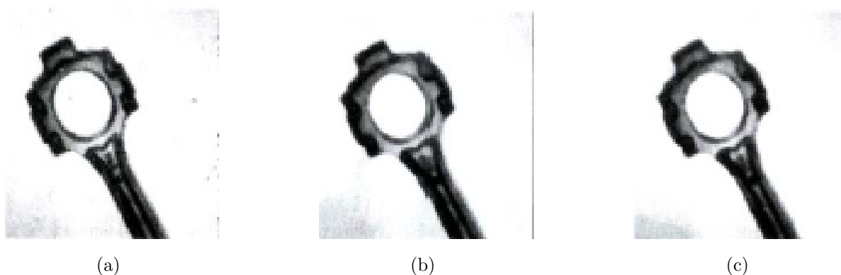
Figure 2.7: Results of 3 \times 3 , 5 \times 5 and 7 \times 7 median filters. source
