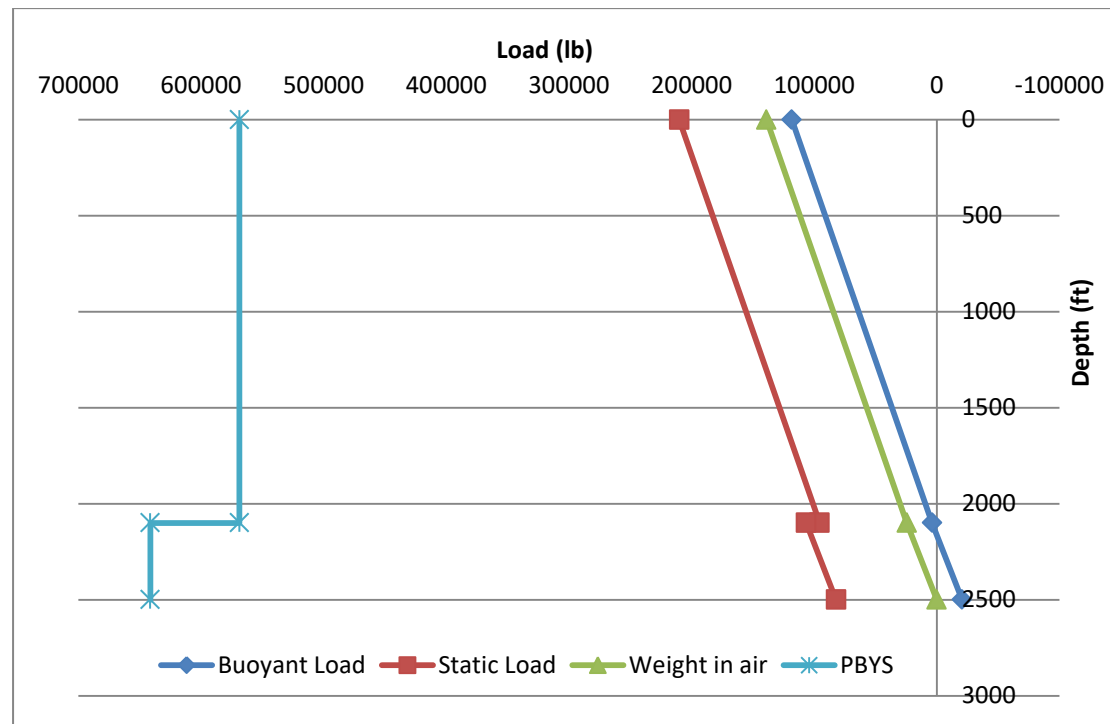
Diagram 8: Tension loads for surface casing.
