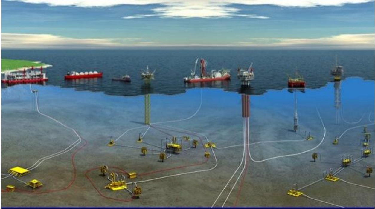
Figure 1-5 : The subsea production system
