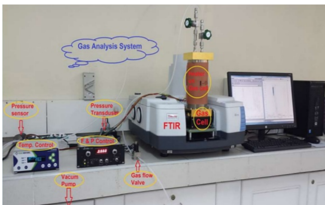
Figure 4.6: A complete FTIR-based gas analysis system
