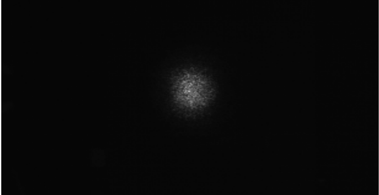
Figure 7.32: The laser beam recorded after reflected on a golden plate obviously the speckle is very intense
