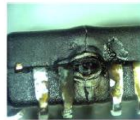
Package Burnt/Cracked
