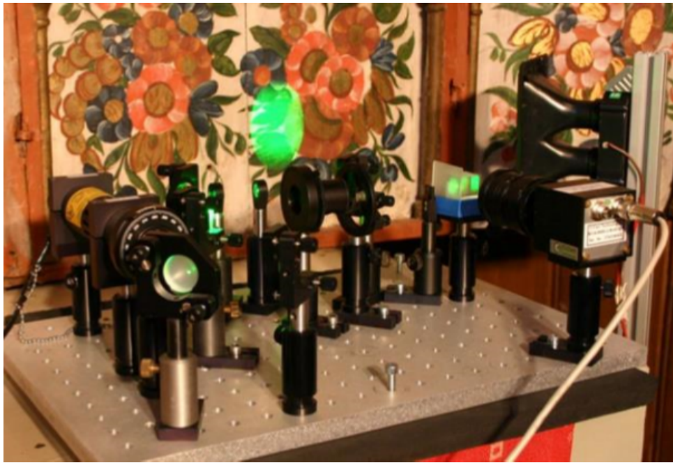
Figure 3.13: Photograph of the Digital Speckle Pattern Interferometry setup with loudspeaker
