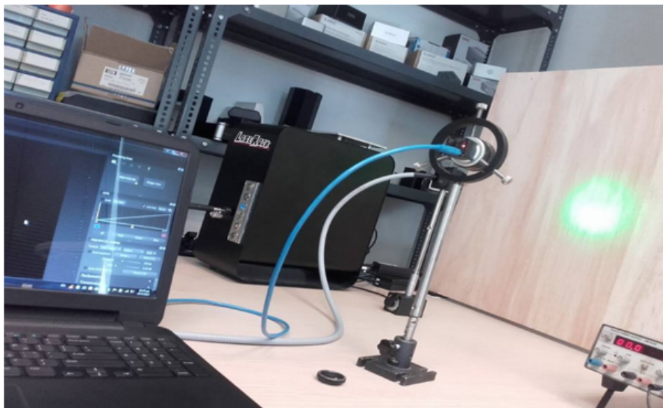
Figure 6.3: Laser Speckle Imager first Setup
