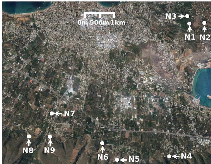
Figure 1.1: City-scale, mesh network topology, tested in this work (with connectivity in Fig. 2.1). Extended area must be served with limited resources (i.e., transmission power and bandwidth). Coloring in 802.11s must be performed judiciously.
