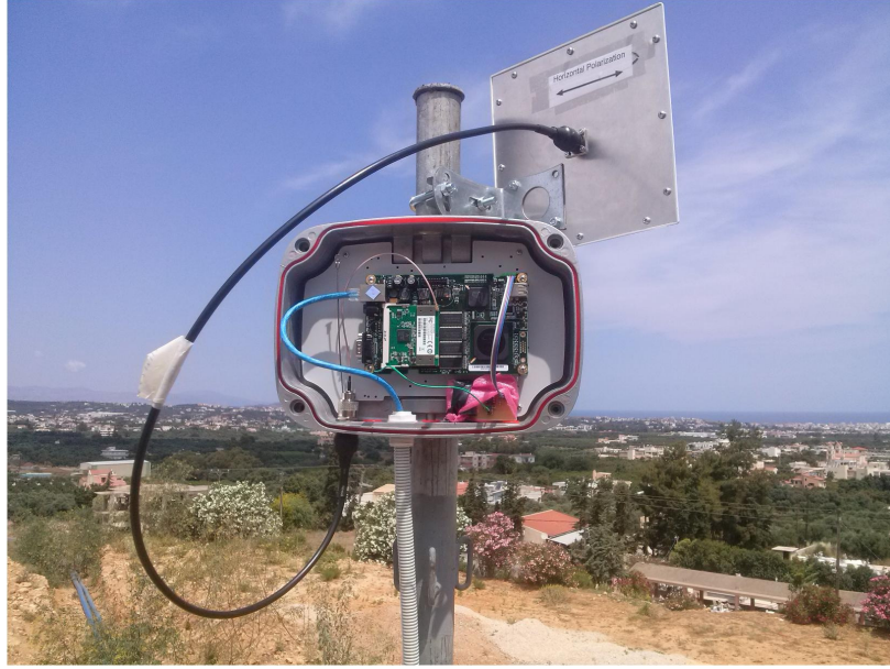
Figure 2.3: ALIX 3D2 in an waterproof case with an antenna attached to a radio interface.
