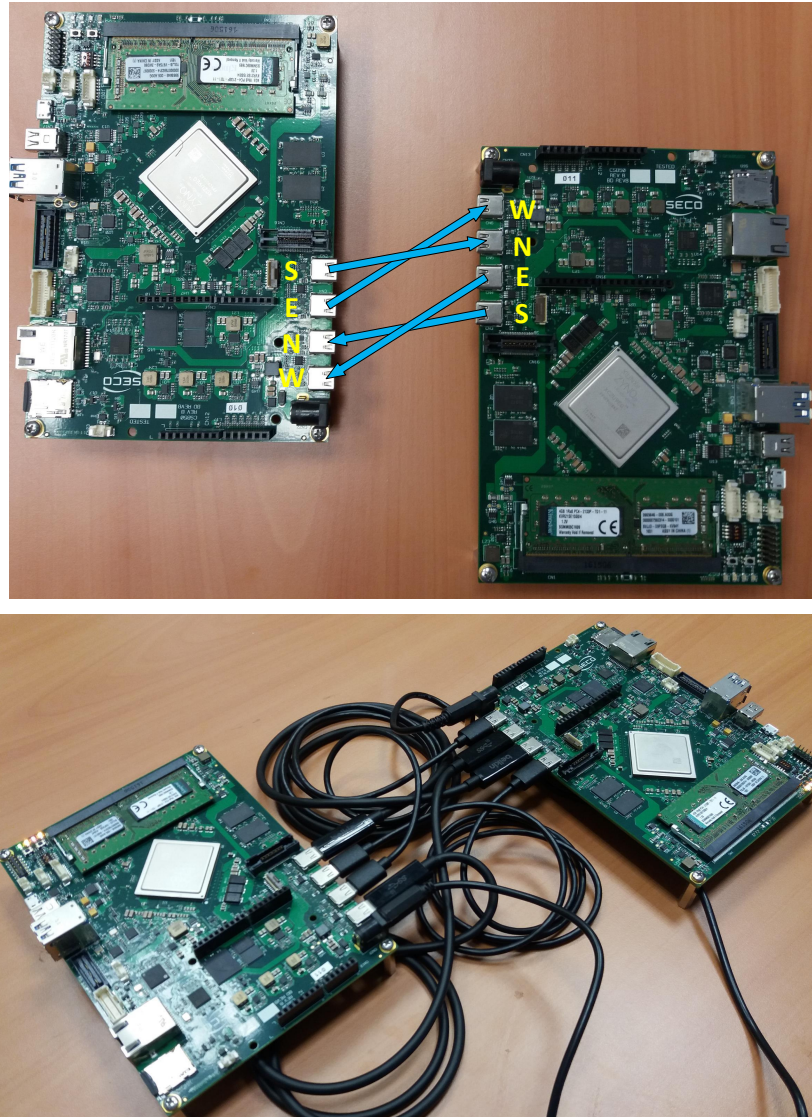
Figure 5.11: Two AXIOM boards programmed using the 3x3 router (for 2-D torus topologies) in 2 independent rings, to utilize all 4 connectors.
