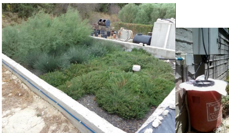
Figure 13. View of the pilot scale HSF-CW (on the left) and the BPA adding set up (on the right).
