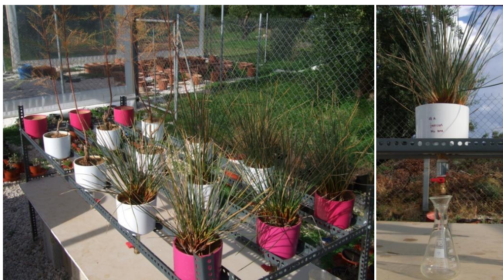
Figure 6. Overview of the pot experiment (left) and details of the pot /sampling port design (right).
