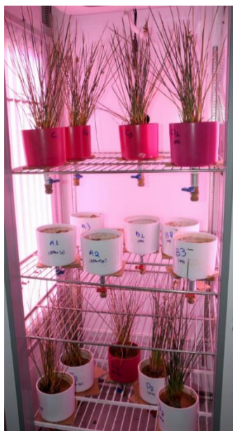
Figure 5: Overview of pot experiment with planted and non-planted treatments in the growth chamber
