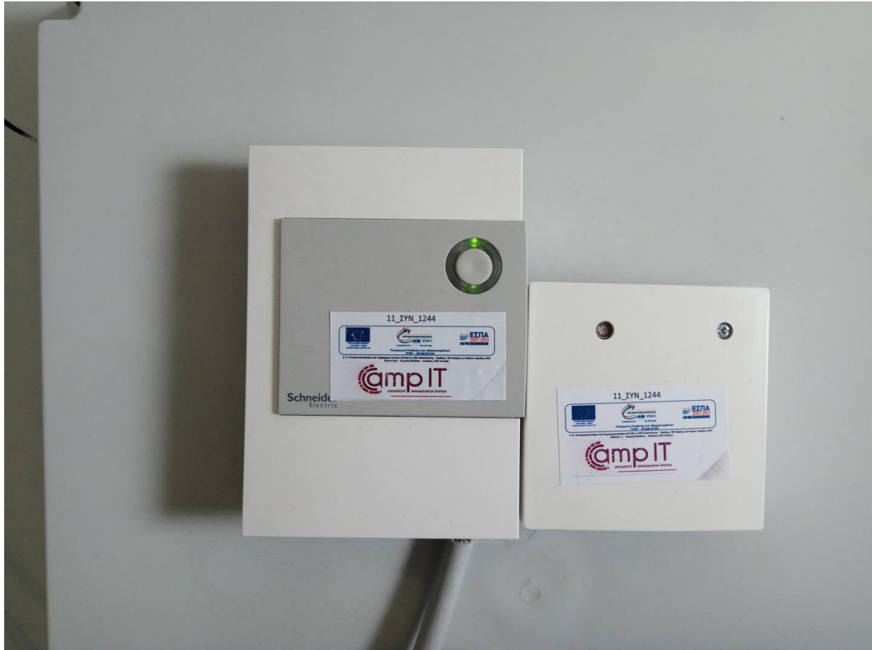
Figure 2.2 light sensor ,CO2 sensor, Humidity sensor (RH) , Thermistor embedded
