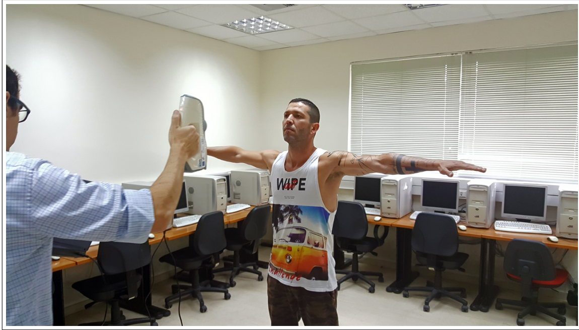
Figure 4.11: Process of white light scanning
