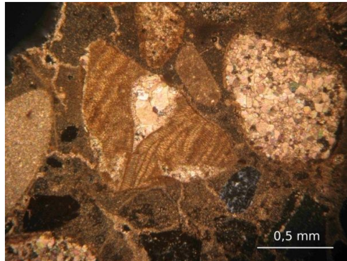
Figure 4.35: Secondary calcite formed around a fossil, possibly providing (supplying) the neighboring cracks with \text{Ca}^{2+} ions.
