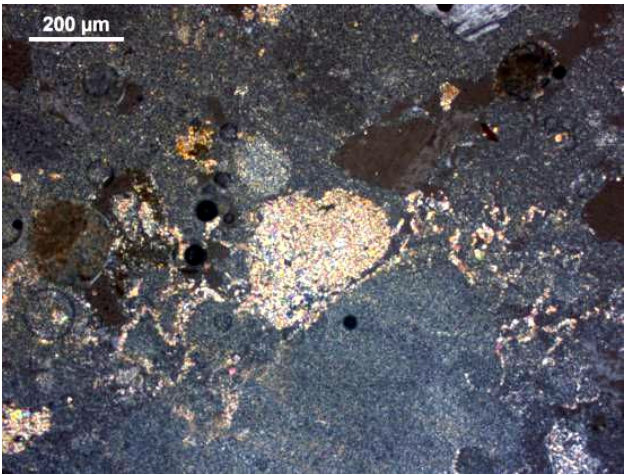
Figure 4.26 (Left): Secondary calcite precipitated around a lime lump XD1
