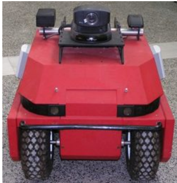
Figure 1 ATRV-mini vehicle in its original form
