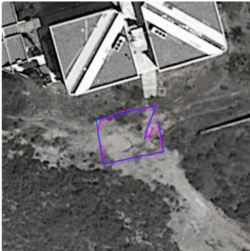
Figure 29 The paths followed by the target object and the robot are marked blue and pink respectively
