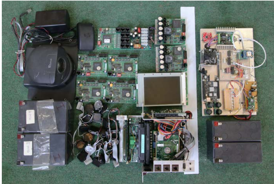
Figure 17 Removed electronics (left side of the line) next to the new ones used (right side)
