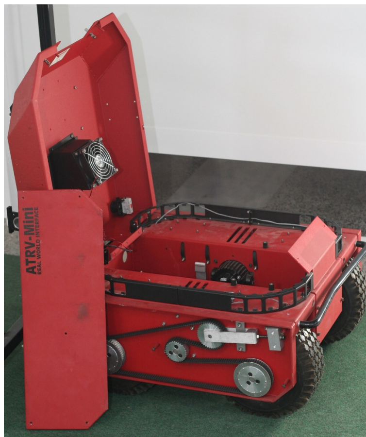
Figure 4 ATRV-mini with the electronics removed
