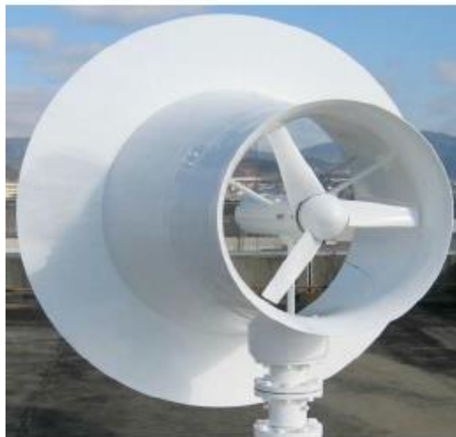
Figure 1.12: 500W wind-lens turbine [Ohy10].
