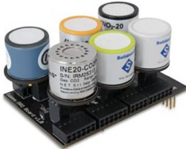
Figure 3.18: Gas Sensor Board
