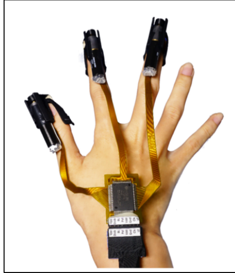
Figure 10. FinGar a finger glove able to provide electrical and mechanical feedback
