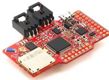
Figure 3.3: Zolertia Z1 board
