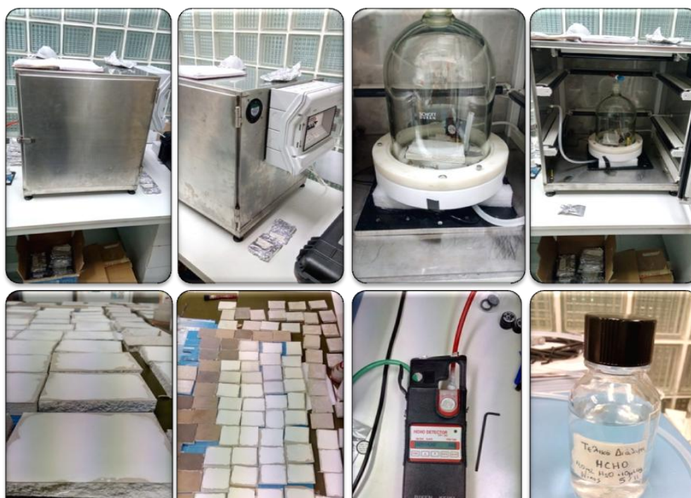
Image 7. Handmade Photocatalytic Apparatus: Aluminum box, Pyrex chamber, BM samples with different coating, HCHO sensor, HCHO solution.
