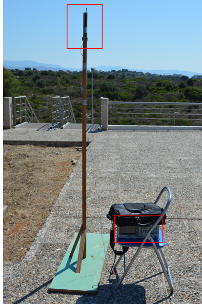
Figure 2.2: ADG1919 switch (top red rectangle) controlled by a Tektronix AFG3021B (bottom red rectangle).
