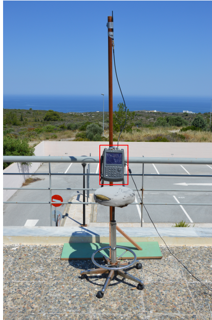
Figure 2.8: Agilent N9912A spectrum analyzer set upped for the experiment.
