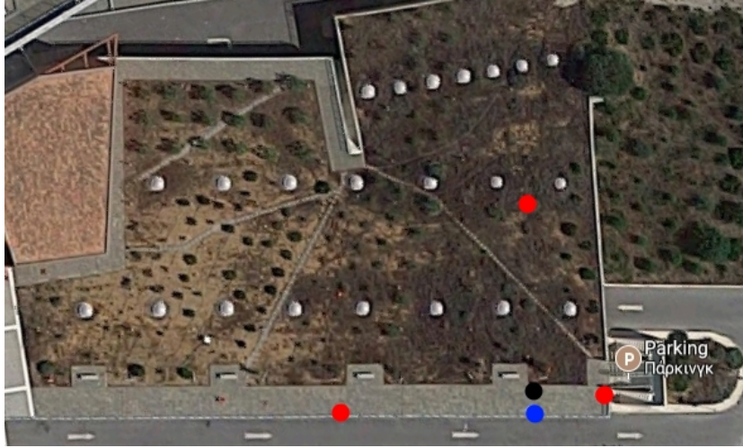
Figure 4.5: First setup from satellite, located at the garden of the ECE department of Technical university of Crete. The red dots are the emitters, the blue dot is the reader and the black one is the tag to be localized.
