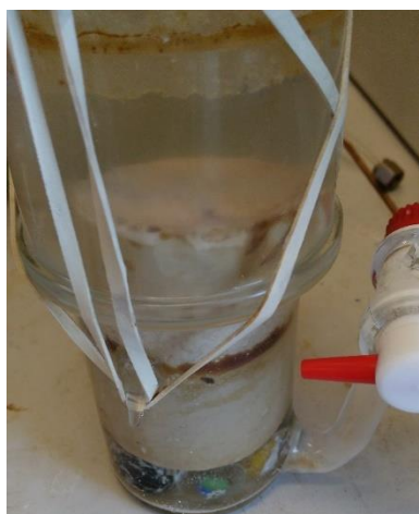
Figure 6.16: Lower part of Spontaneous Imbibition cell
