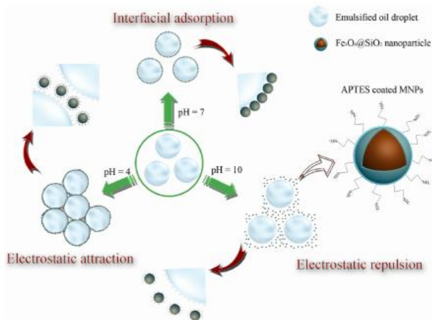
Figure 160 - Interaction mechanism between APTES coated magnetic nanoparticles for the resolution of oil in water emulsions (Lu et al. 2017a)
