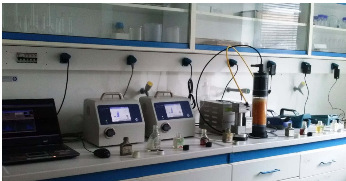
Figure 4.1. Testing of experimental setup for emission from painting materials.
