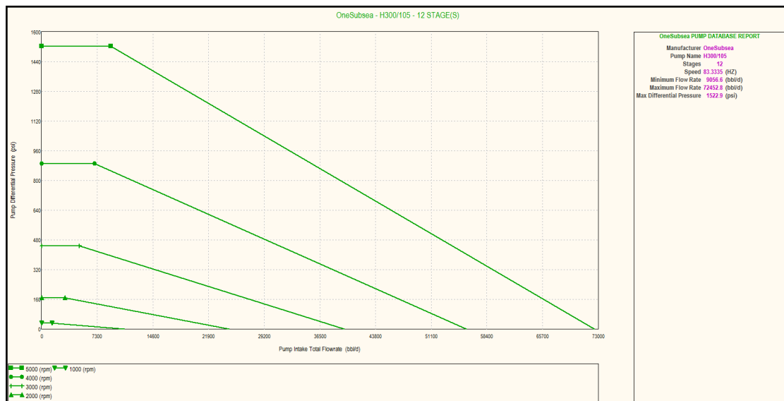
Figure 67: Pump's data and characteristic curves for different speeds.
