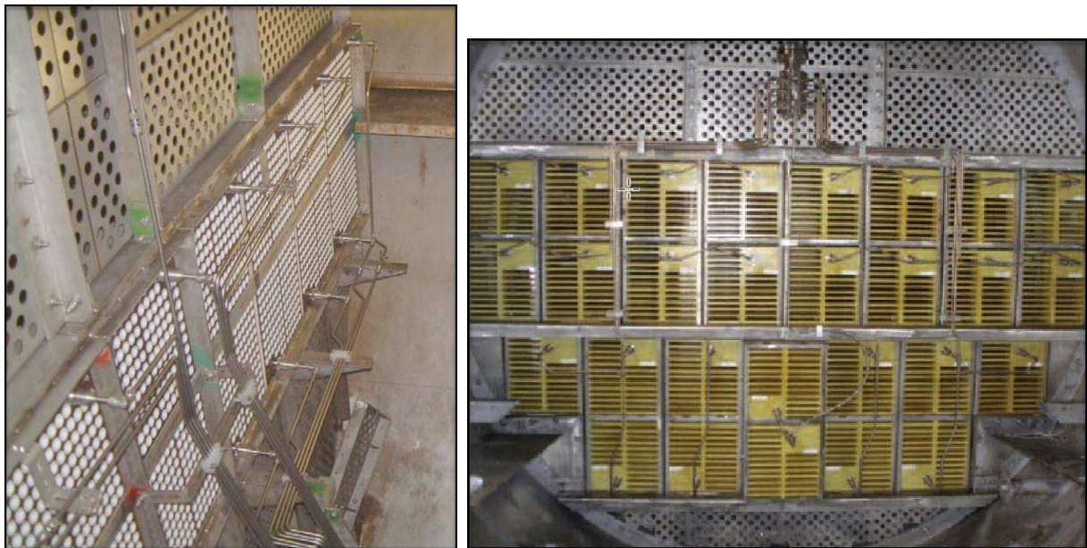
Figure 78: VIEC wall installed in 1 st stage separator with tubular flow channels (left), Advanced Electrostatic Internals in the 1st Stage Separator Enhance Oil/Water Separation and Reduce Chemical Consumption on the Troll C Platform, Erik A. Wolff/ABB Offshore Systems, Trond L. Knutsen/Norsk Hydro, Wojciech Piasecki/ABB Corporate Research, Peder Hansson/ABB Offshore Systems, Pål J Nilsen/ABB Offshore Systems, OTC 16321, 2004, [145], VIEC installed in a separator with rectangular flow channels (right), image source: http://www.hamworthy.com , Electrostatic phase separation: A review, S. Mhatre, V. Vivacqua, M. Ghadiri, A.M. Abdullah, M.J. Al-Marri, A. Hassanpour, B. Hewakandamby, B. Azzopardi, B. Kermani, Chemical Engineering Research and Design, 2015, [97]. In both cases perforated baffles are placed above and below the VIEC electrocoalescer.
