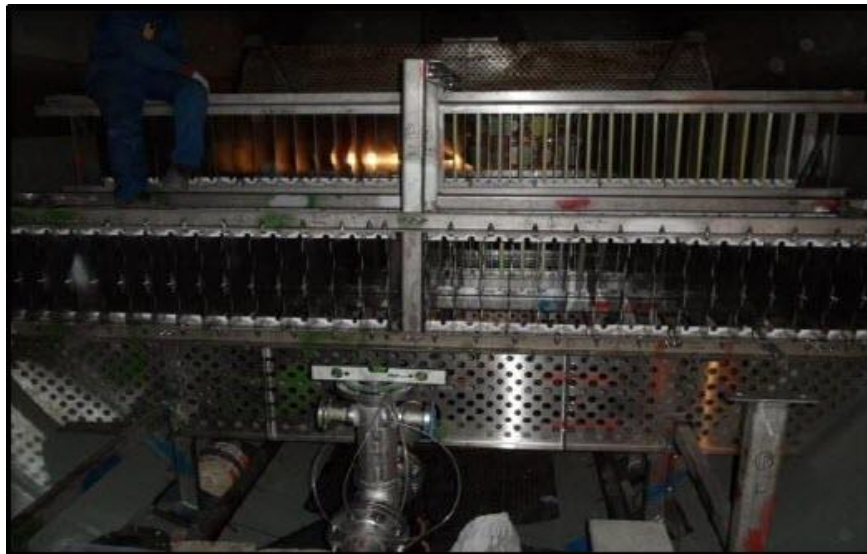
Figure C9: VIEC LW electric sheets installed in 13-V-4001 vessel, Vessel Internal Electrostatic Coalescer Technology (VIEC), SPE 156087, Ali AlQahtani, Qatar Petroleum, 2012, [240].
