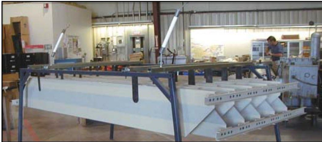
Figure 72: Array of composite electrodes. The conductive region in the middle is surrounded by the non conductive material, Compact and lightweight equipment for floating production systems, Erik Sellman, Pavan Mandewalkar, Gary W. Sams, Cameron Process and Compression Systems, OTC-24727-MS, 2014, [104].
