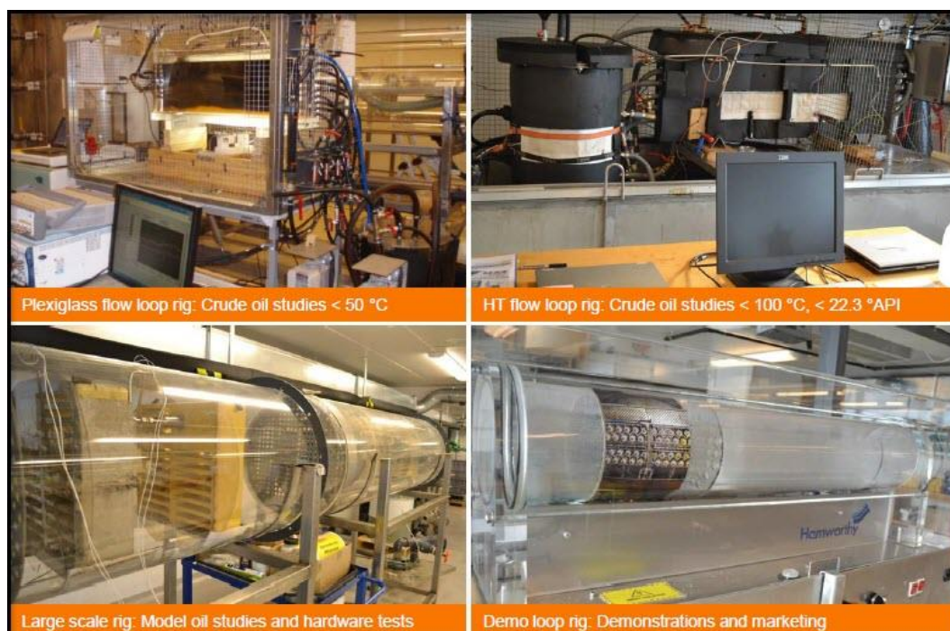
Figure 87: Laboratory multiphase platform, Electrostatic Destabilization of water-in-oil Emulsions: Use of laboratory scale experiments to debottleneck and optimize separation processes , Erik Bjørklund, Toulouse Workshop, 2012, [153].
