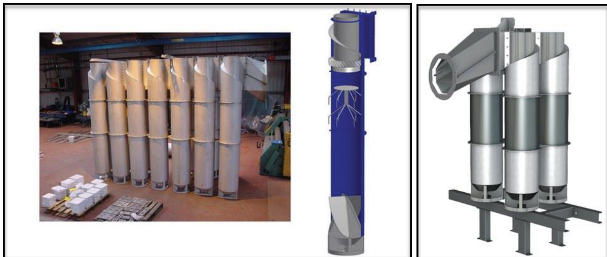
Figure B5: Inlet cyclone with turbine blades, internal vortex tube, gas blocking plate and liquid antispin blades (Photo courtesy of FMC Technologies), Savvy Separator: Design of Cyclone Separators: Internals and Liquid Levels , Robert Chin, Padden Engineering , 31 May 2015, OGF Vol.4 Issue 3 , [258].
