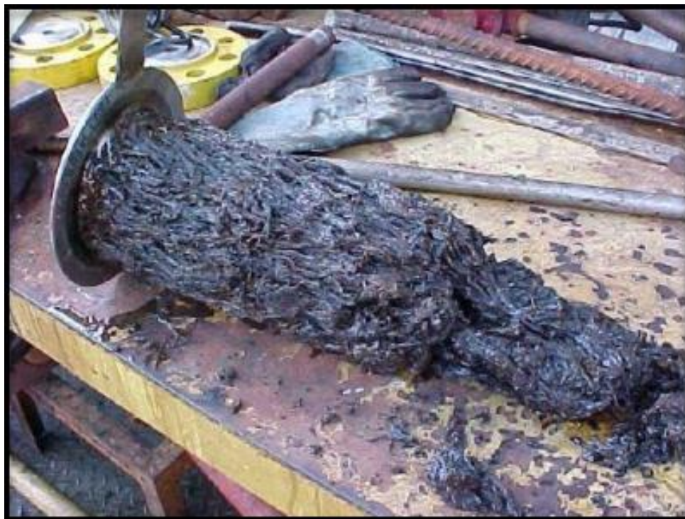
Figure 21: Naphthenate deposit found in an electrical desalter in Angola (source: www.oilfieldwiki.com )
