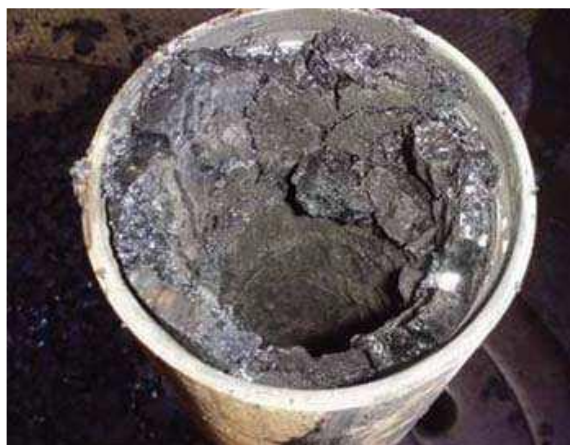
Figure 18: Asphaltenes clogging a pipe. Courtesy of A. Pomerantz, Schlumberger (chapter 2 Petroleum Asphaltenes Lamia Goual University of Wyoming USA) [37].
