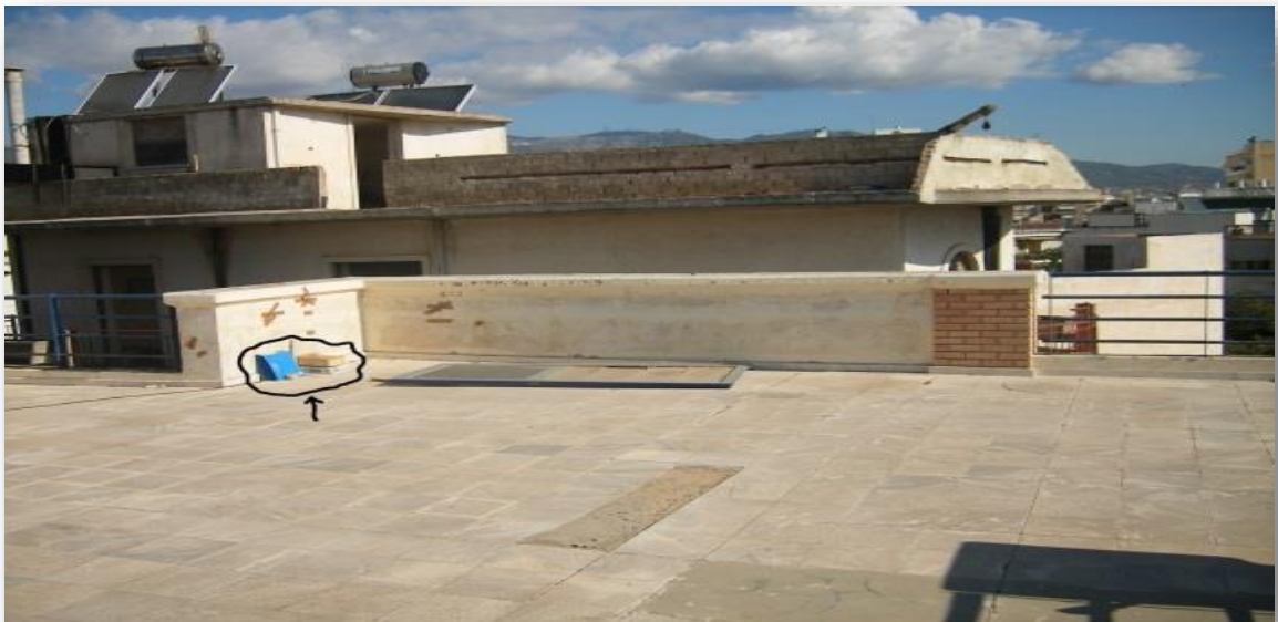
Figure 23 Positioning of the K type thermocouples # 1 positioning (black circle) in the 3 rd floor's roof
