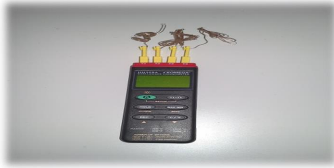
Figure 21 Omega HH309 data logger and K type thermocouples
