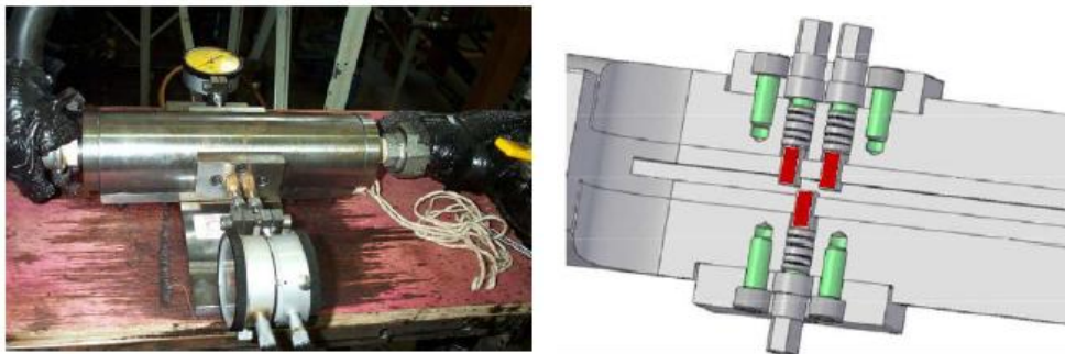
Figure 88: A duct with a square cross section and three movable drawers. [71]
