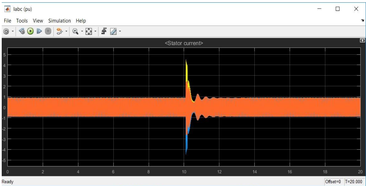
Figure 8.31: Stator Three Phase Current Characteristics of Hydro Power Plant in Kastraki with transmission line fault at 10.1 s with PID for 0.8866 pu (in y pu and in x-Axis Time in s)-A3
