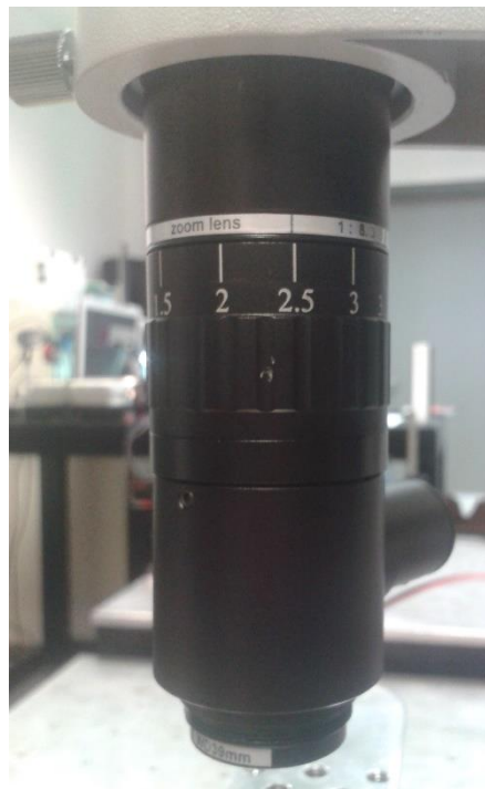
Figure 3.4: Magnification values on the parfocal lens
