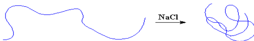
Figure 5.5: Salinity discharges the polymer chains which results in their random configuration
