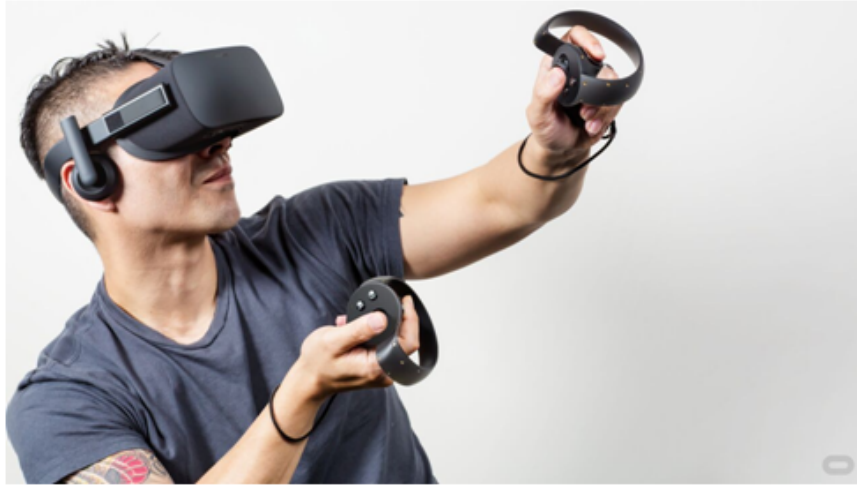
Figure 2.5: wireless controllers with hand-tracking capabilities.
