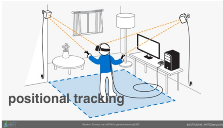
Figure 2.2: positional tracking
