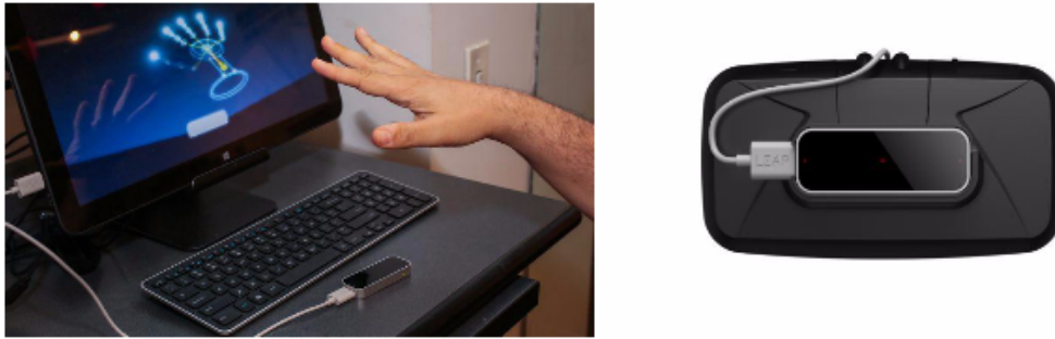
Figure 6.1: Leap Motion controller. Left: controller placed on desk facing upwards. Right: controller mounted on HMD facing forward.
