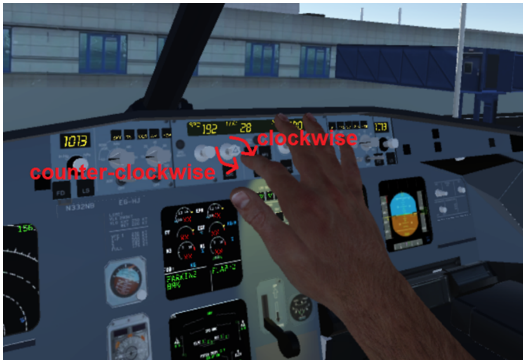
Figure 6.5: Making a circle with the index finger as shown in the image will be recognized as a gesture.
