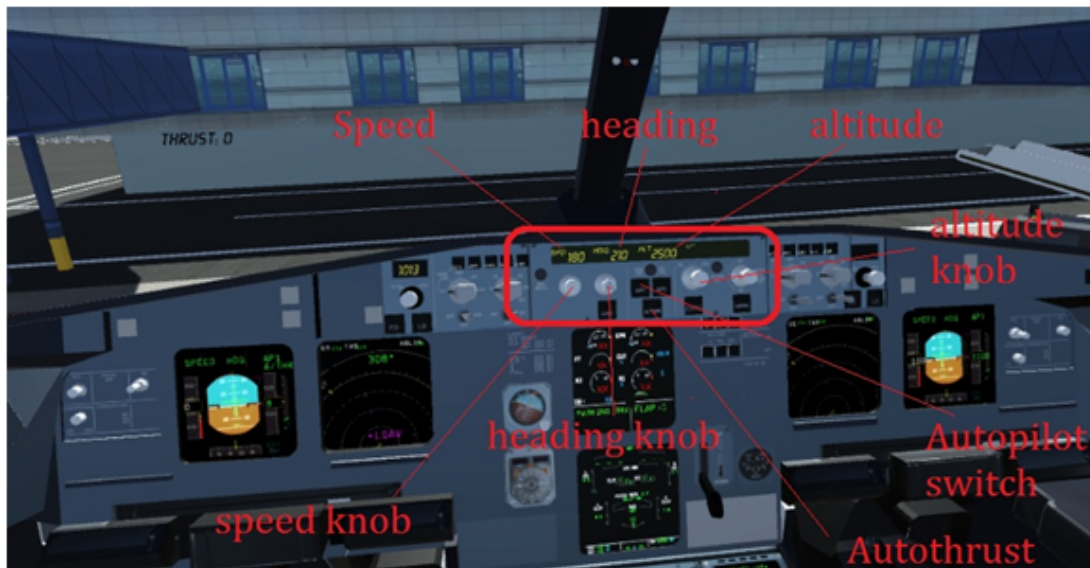
Figure 5.18: Autopilot: LCD displaying current target airspeed, heading and altitude, and rotary knobs
