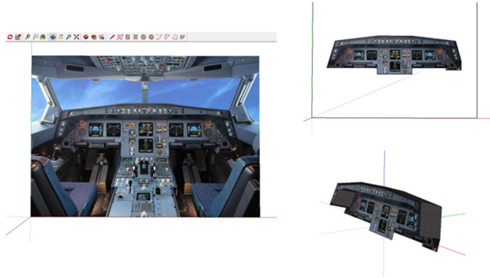
Figure 5.2: Making the 3D model based on a photograph in SketchUp
