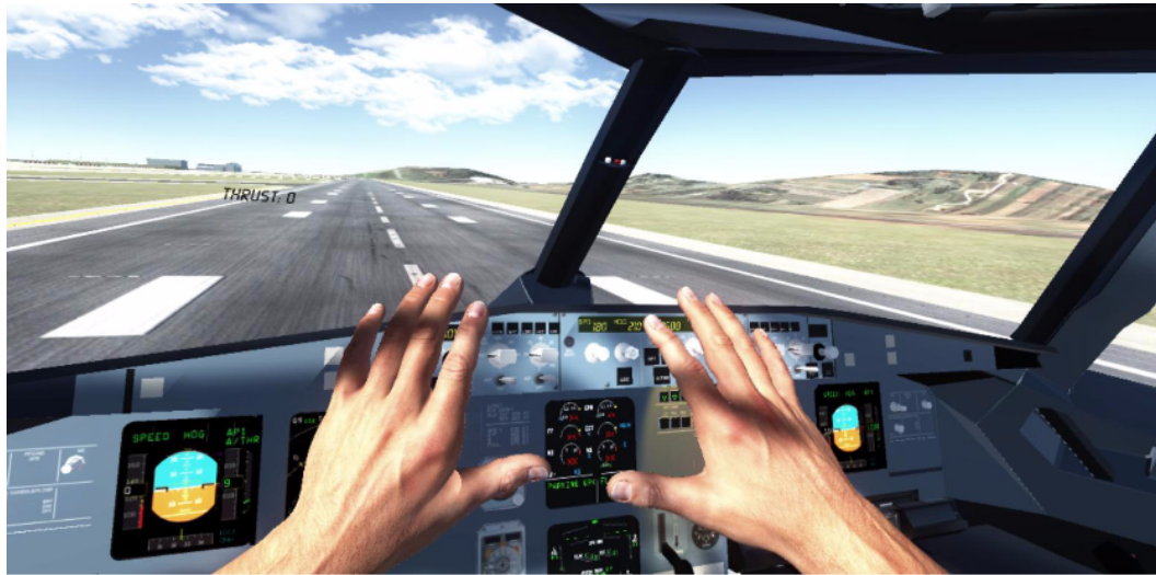
Figure 6.3: Leap Motion’s realistic hand models in real-time gameplay
