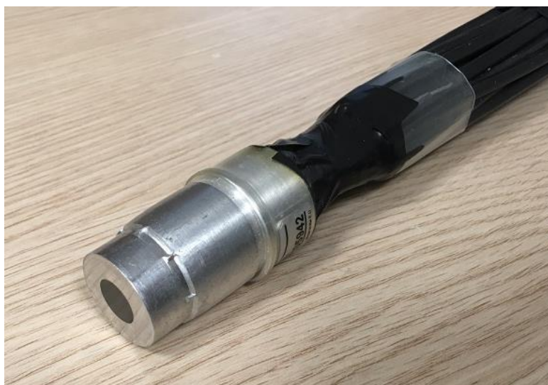
Figure 111 – Fiber Optic Bundle
