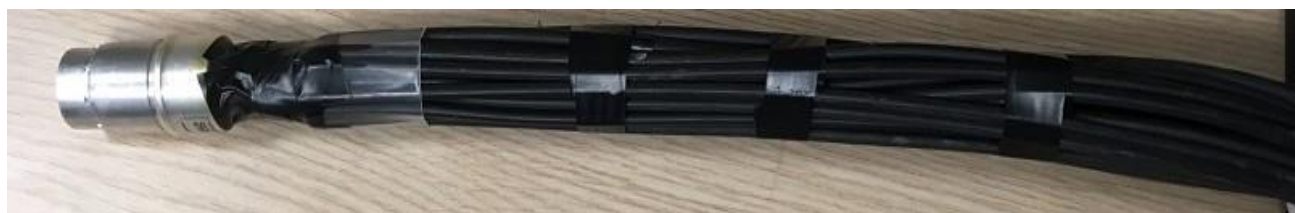
Figure 114 – Fiber Optic Bundle and LED Board Coupling
