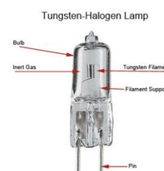
Figure 12 | Outline of halogen lamp
