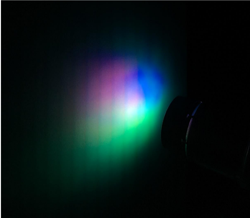
Figure 121 – Image by reflection of three LEDs (RGB) at the fiber optic bundle end
