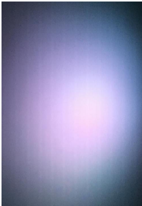
Figure 126 – Image by reflection of three LEDs (RGB) at the diffuser's output
