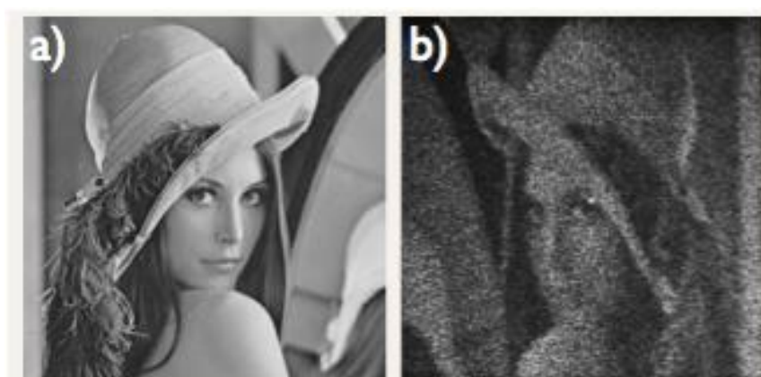
Figure 163 - a) Input image is fed into a display system b) Image with laser speckle noise, which could be an image that is displayed by a laser projector.
