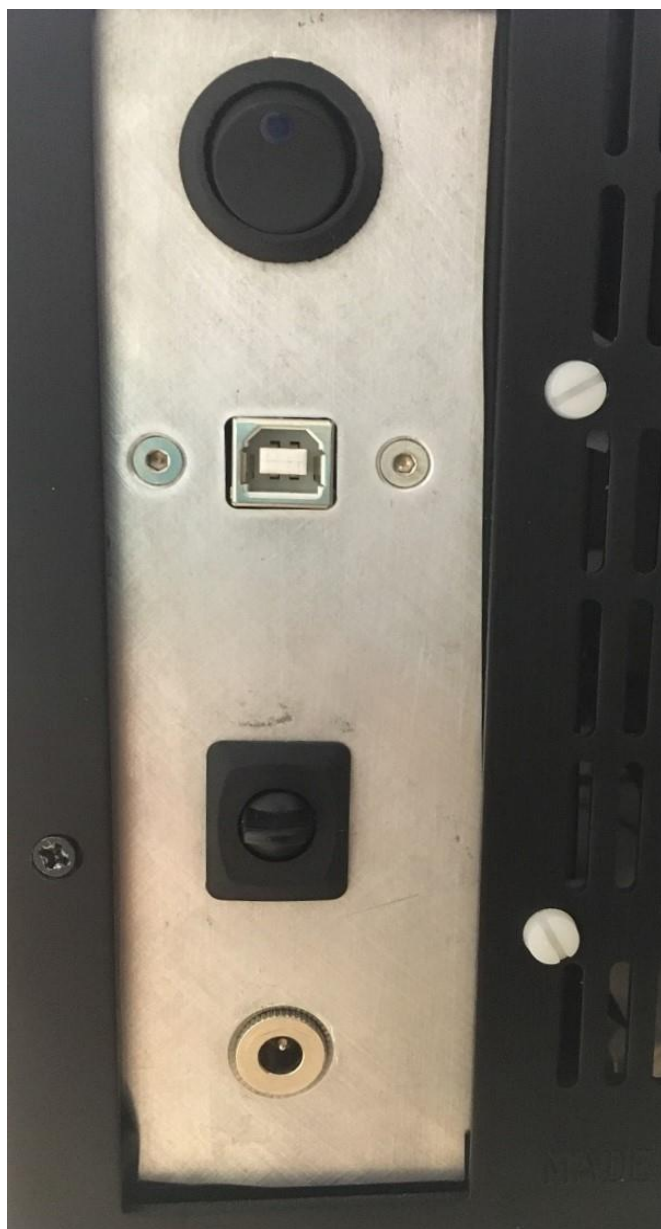
Figure 169 – Front panel and Rear panel. In the front panel the push buttons that control the laser diodes in non-USB mode are located. Looking at the rear panel, there is the central switch, the USB port for connecting with the PC, the rocket switch with which push button control or USB control of the laser diodes is selected, and the power jack.
