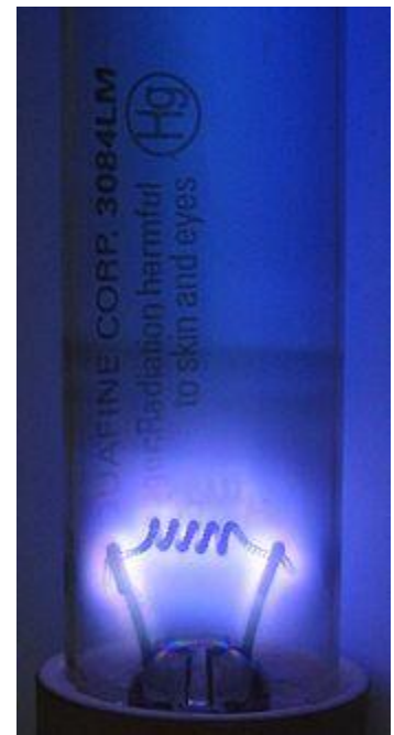
Figure 17 | Glow of a germicidal lamp excited by a high voltage probe.
