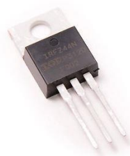
Figure 148 – Power MOSFET IRFZ44N
