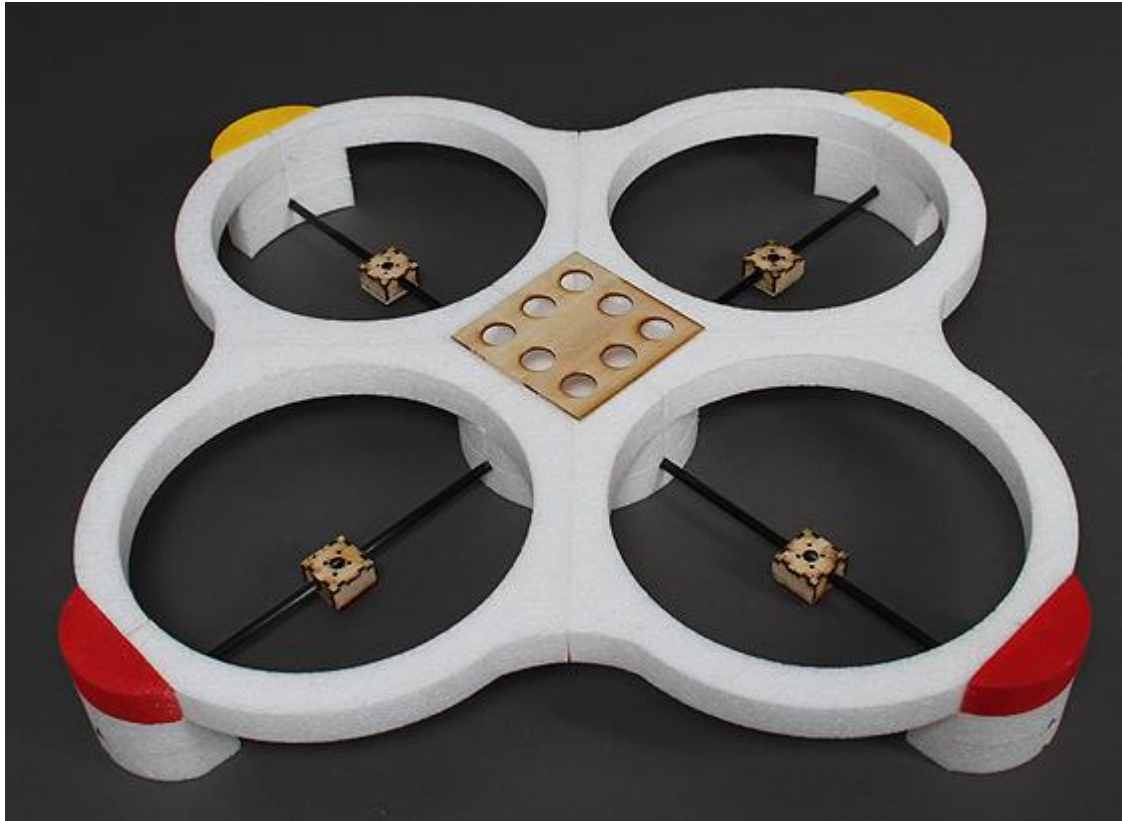
Figure 0.2 EPP quadcopter frame in full assembly. Under the wooden cap there is room for the PDB and ESCs. The wooden boxes provide a base for the motors. (HobbyKing, 2015)
