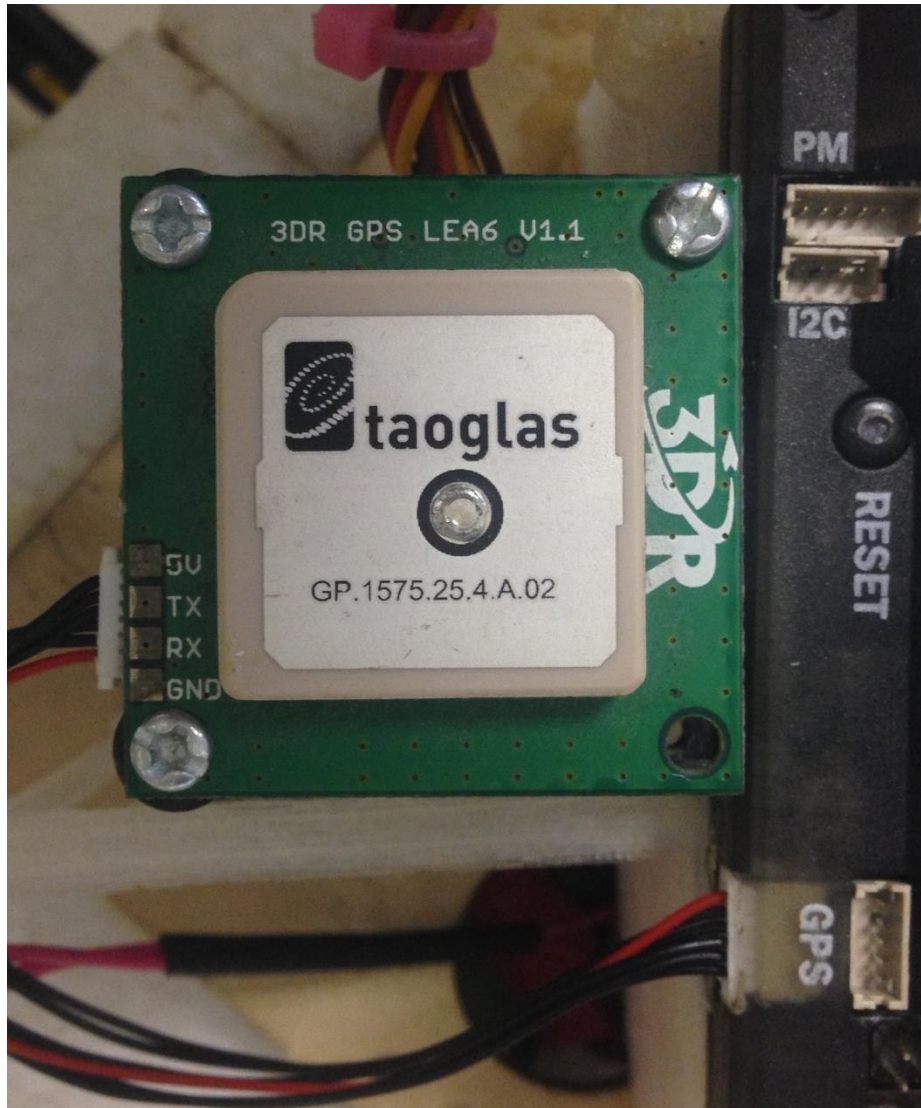
Figure 0.4 3DR's GPS LEA-6 v.1.1 mounted on the foam quadcopter, next to the APM2.5 autopilot.
