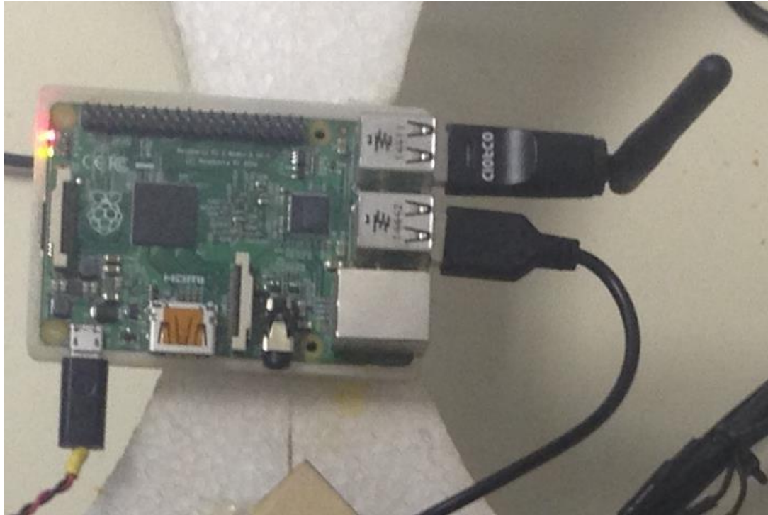
Figure 0.5 The Raspberry Pi 2 model B with the Odroid Wi-Fi module installed, as part of the full assembly of the foam quadcopter. It is powered by one of the 5V outputs of the autopilot through a micro-USB port.
