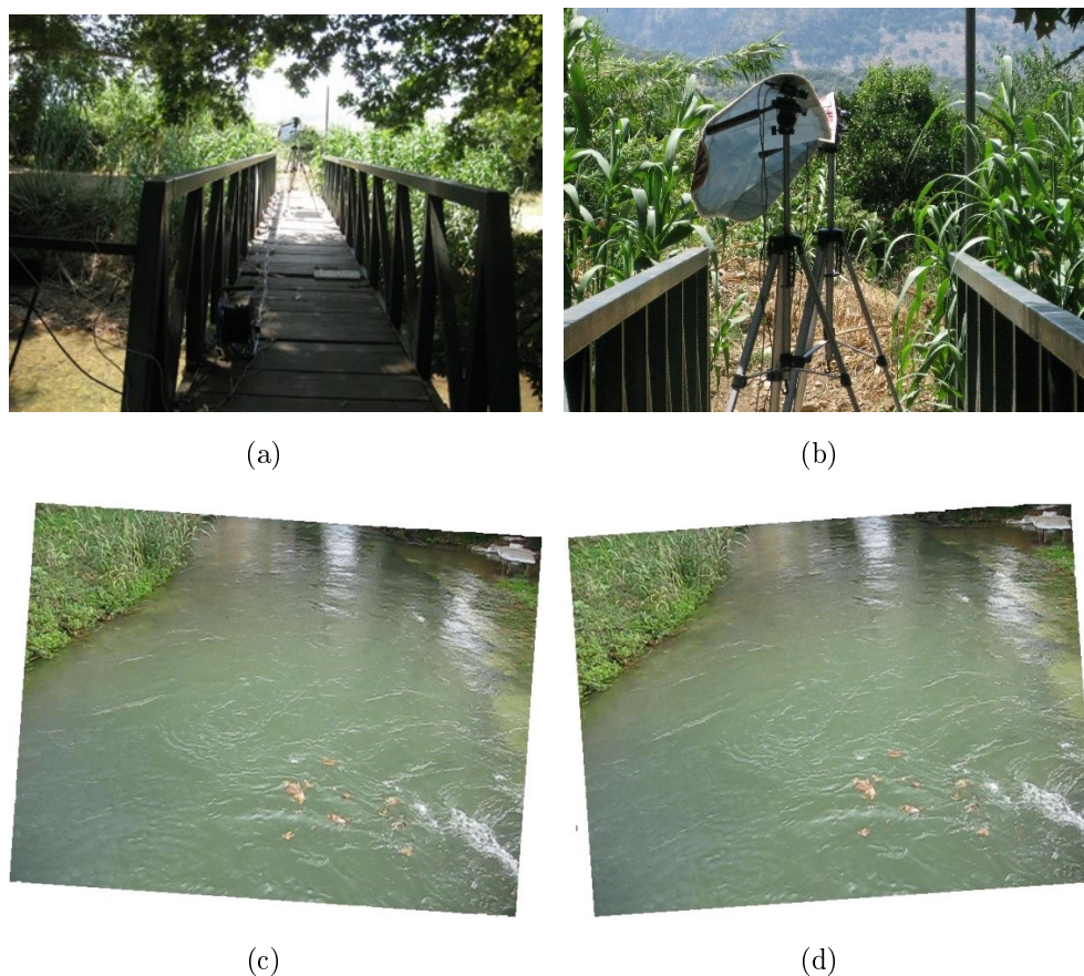
Figure 5.9: Koiliaris River site, (a) The convergent stereo rig placement on top of the bridge, (b) Close up on the stereo rig used, consisting of two CCD cameras, (c) View of the Left camera, (d) View of the Right camera without rectification.
