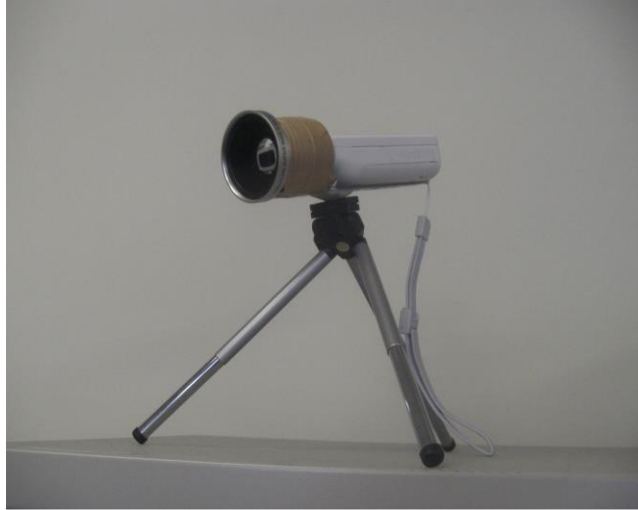
Fig. 5.1 Viewing range expansion by using wide-angle lens [32].
