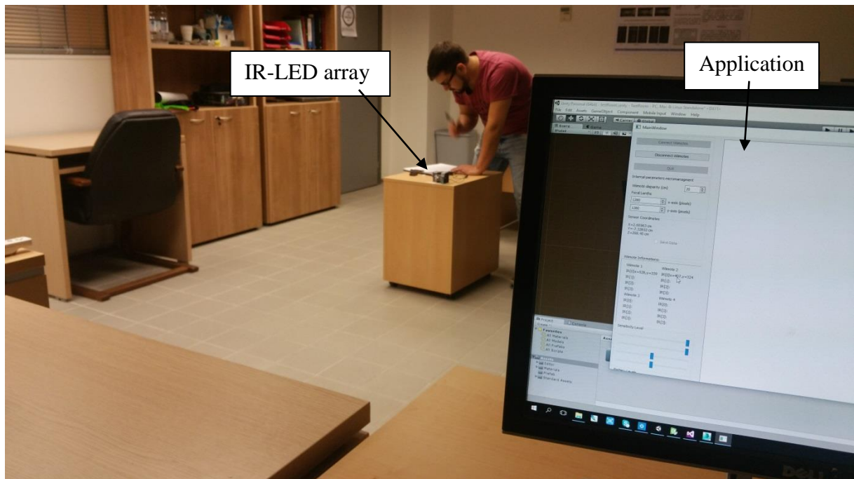
Fig. 4.3 Gathering data in the experiment environment: the IR-LED array on top of a roller table (middle) and the software developed (right).
