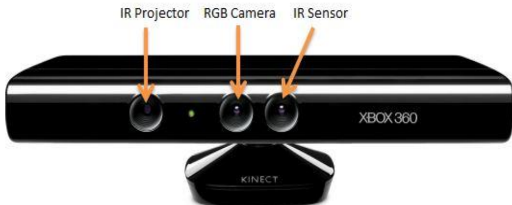
Fig. 2.13 Kinect Device: the IR projector emits a grid of IR light in front of it; this light then is reflected, by objects on its path, back to the IR sensor [12].
