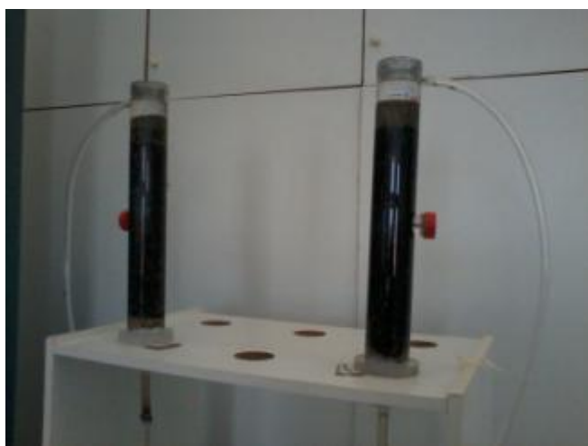
Fig. 5. Pe20Phe and Sd20Phe (left to right) (Plexiglas columns Height/Diameter: 45/5 (cm/cm); biochar: quartz sand 50:50 (v/v); initial phenol concentration 20 mg·L -1 )
