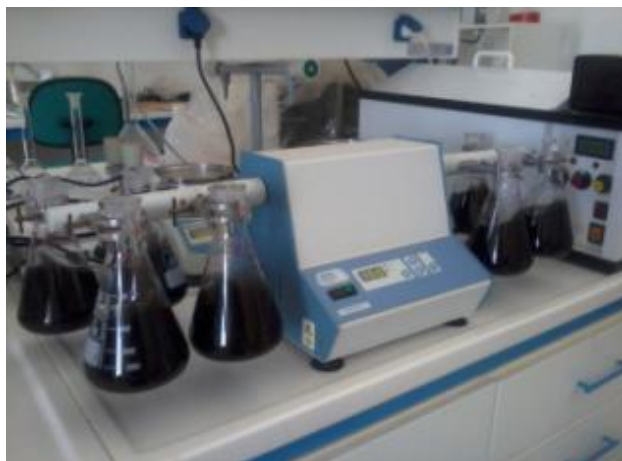
Fig. 2. Vibromatic rocking mixer for shaking conical vials in all experiments
