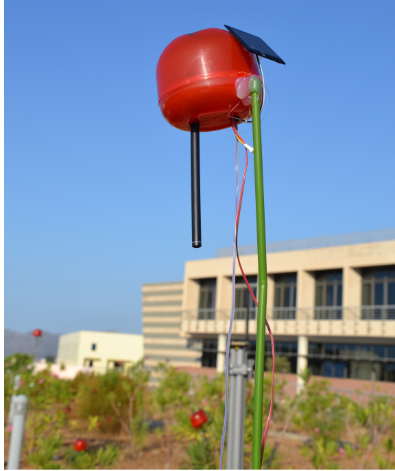
Figure 3.4: The scatter sensor node in the tomato casing.
