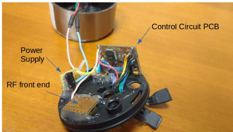
Figure 3.9: A close up of the node electronics. The supercapacitor is not present in the photo.
