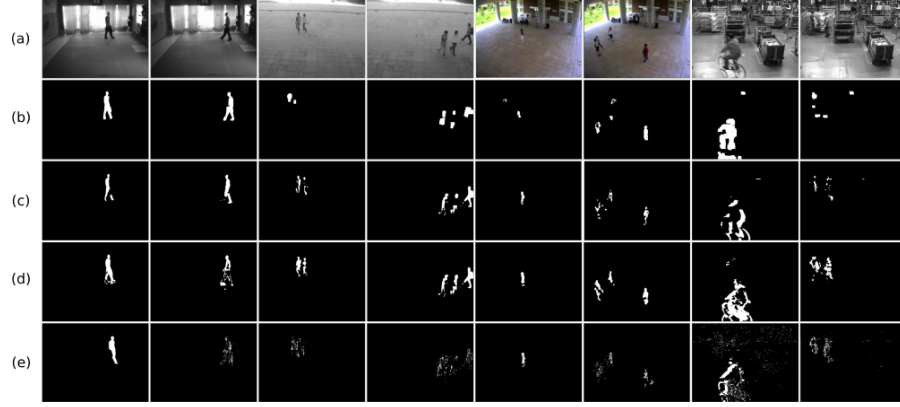
Figure 3.7: (a) Original captured frame, (b) ISL performance, (c) ASMM performance, (d) nPBG performance and (e) GMM performance.
