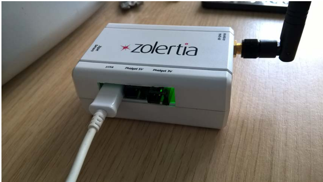
Figure 4.3: A Zolertia Z1 mote
