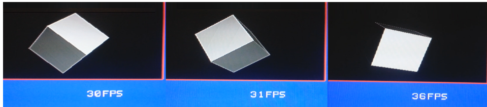
Figure 89: Gouraud Shading phase running on the FPGA
