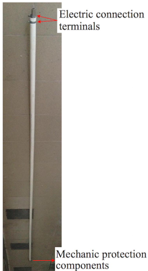
Figure 5.5: The prototype of the TDR-based water level sensor before the installation in the water tank of Ag Mathaios.
