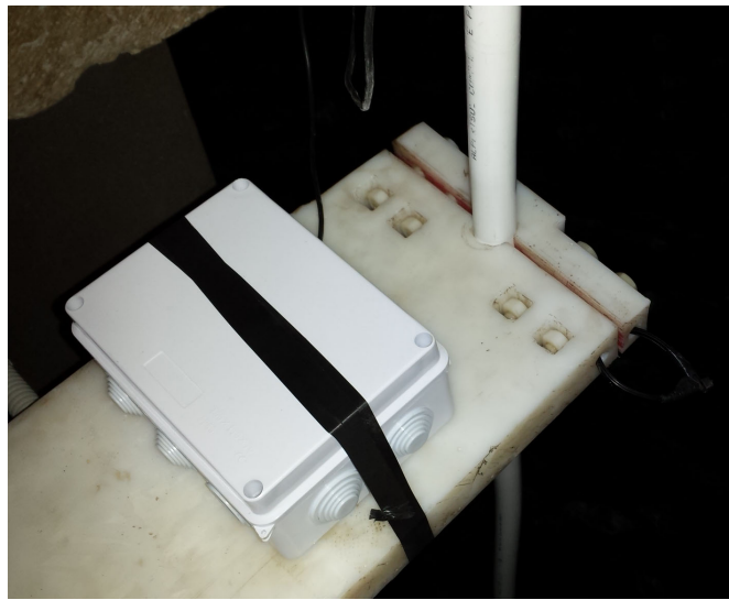
Figure 4.6: The capacitive sensor circuit installed next to the sensor probes in Ag. Iwannis water tank.
