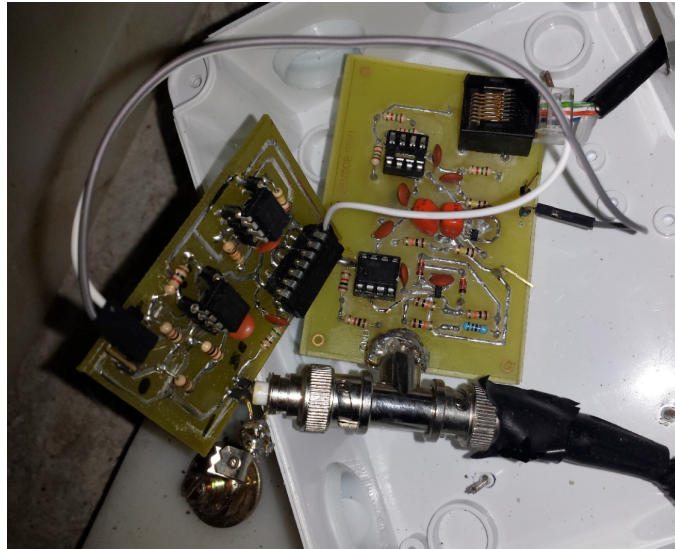
Figure 4.10: The TDR-based circuit boards connected on operation.
