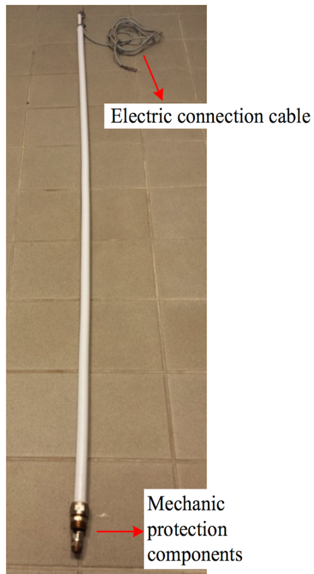
Figure 4.4: Experimental prototype of 2 meter length.
