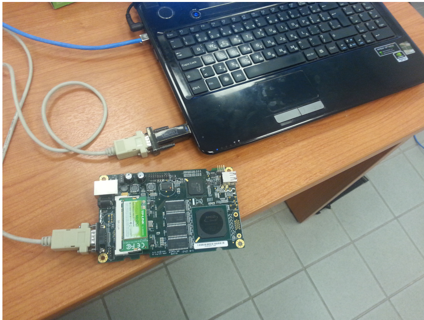
Figure 4.11: Alix Board Connected to a Linux Machine.
