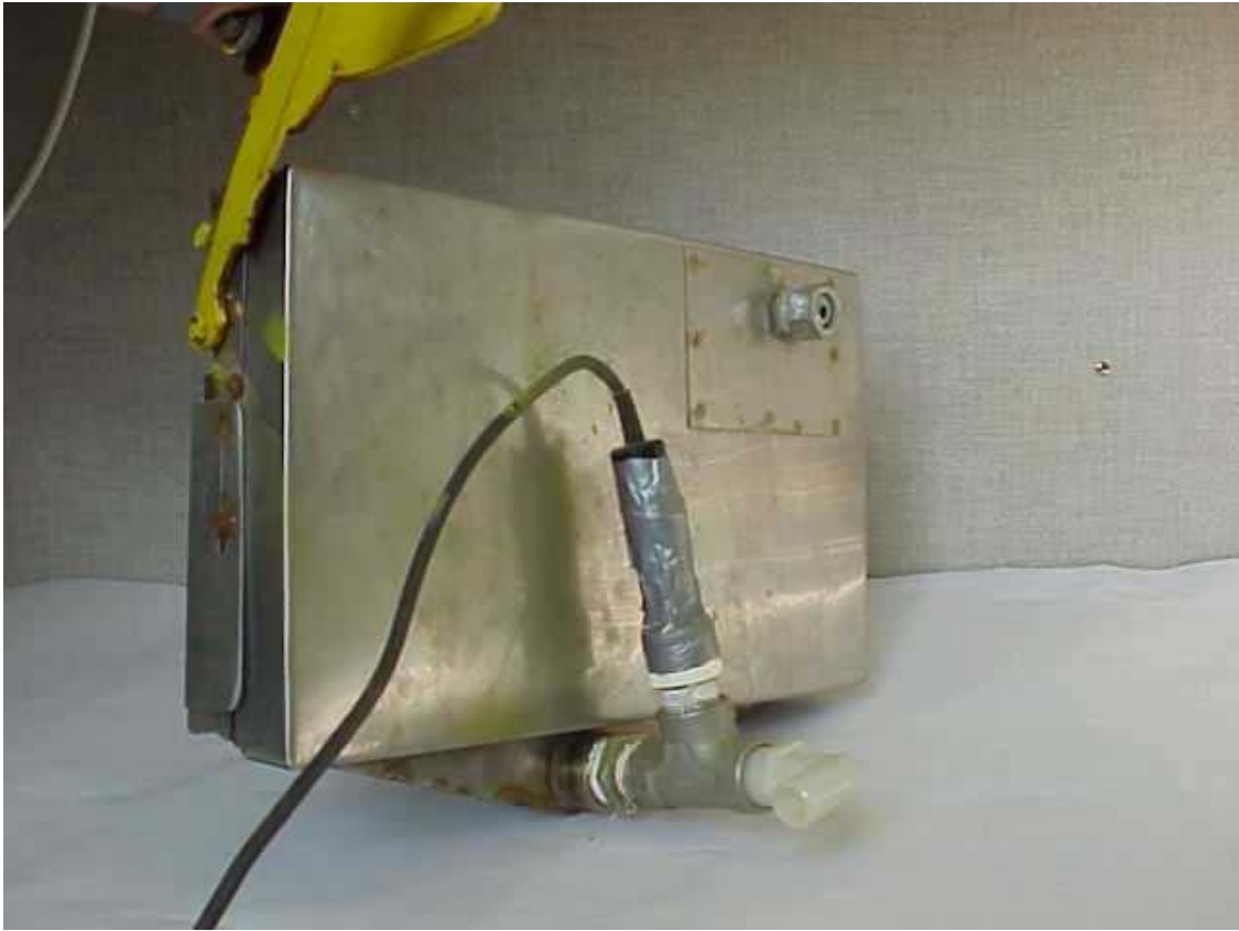
Figure 2-7. Rear View of Collection Device Showing Conductivity Probe
