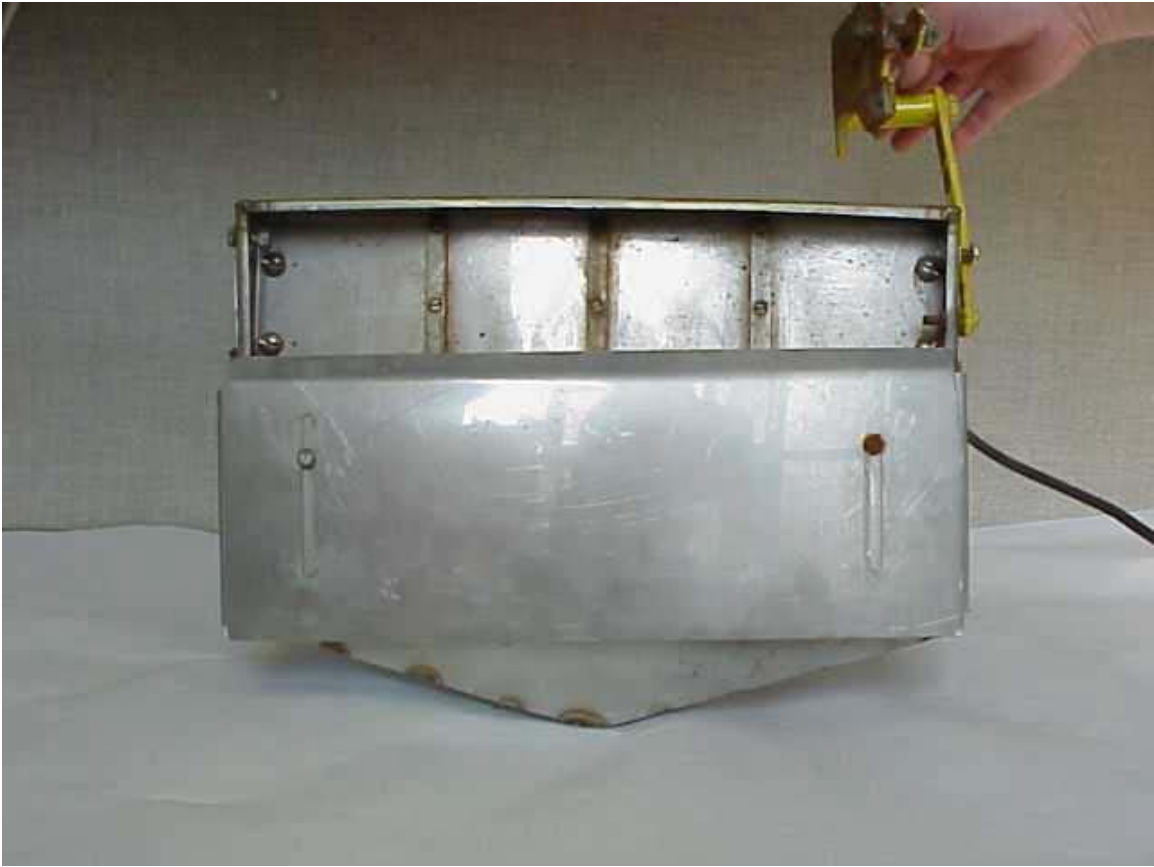
Figure 2-6. Front View of Collection Device Showing Inlet for Tire Spray
