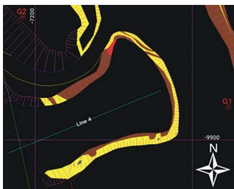
FIG. 6. A part of the geological map (Fig.1) of the quarry and the location of ERT line 4. Red colour indicates the schists (bedrock).
