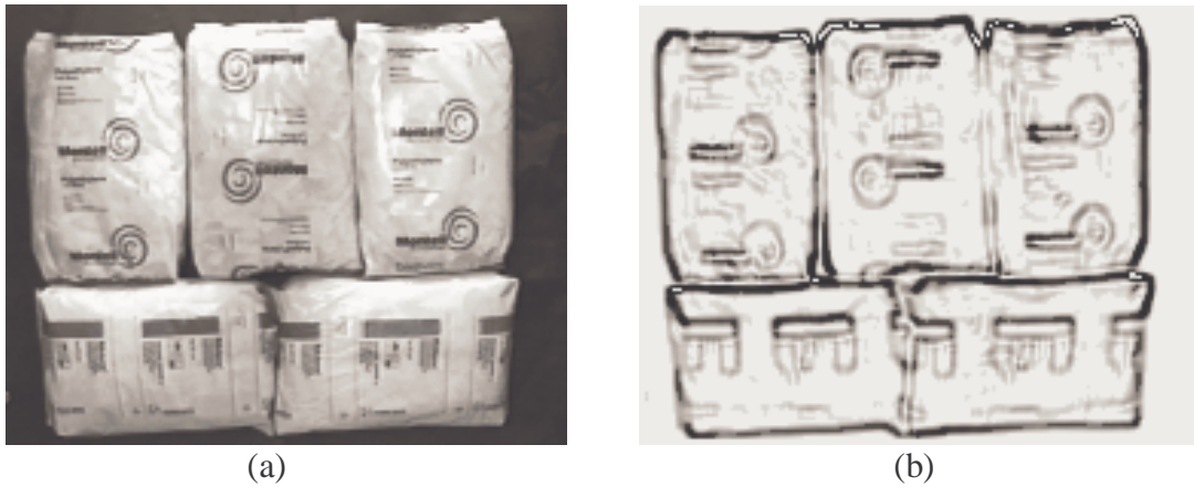
Fig. 5. (a) A pallet layer, (b) the detected edges
