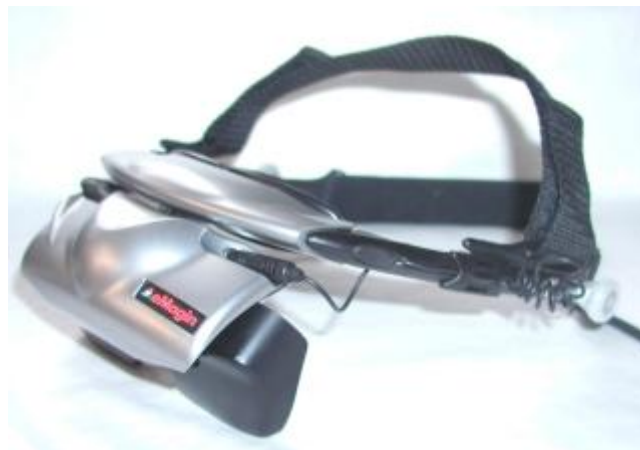
Figure 22. A HMD with a separate video source displayed in front of each eye to achieve a stereoscopic effect
